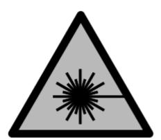
Do not direct the laser beam at persons or animals and do not stare into the direct or reflected laser beam yourself. You could blind somebody, cause accidents or damage your eyes.
