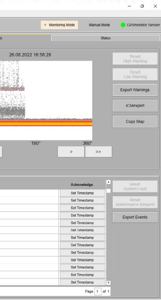
The service software visualises the current readings of the installed PD sensors and indicates partial discharge events or system notifications. It features analysis and reporting functions, such as the display of trending information and phase-resolved PD patterns as well as automatic report generation.
