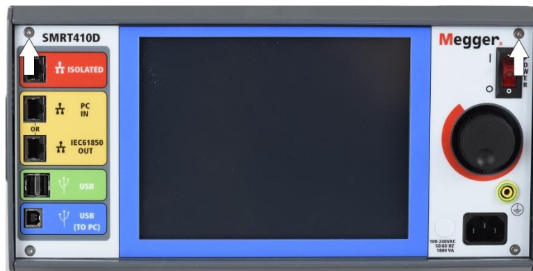
Figure 329 Front Panel Screws, Removal of Top Cover
