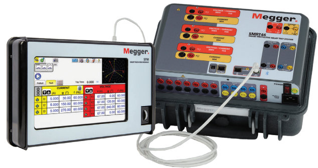
Figure 1: SMRT46 unit with STVI
