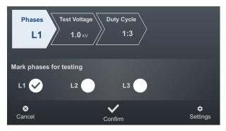
All required measurement parameters and their current values are displayed at the top of the screen, with the segment of the currently active measurement parameter marked in colour. Once this has been set as desired, confirm the setting with to proceed to the next step. The respective segment can be tapped to jump directly to one of the measurement parameters at any time during the workflow if, for example, a previously made setting needs to be adjusted.
