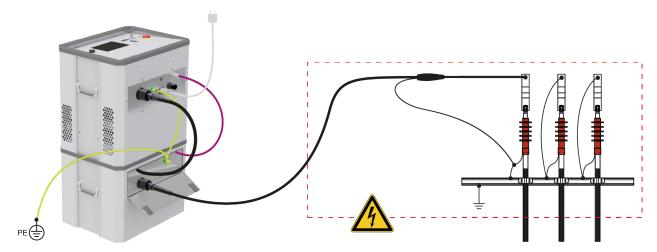
To connect the test system to the test object, proceed as follows:
