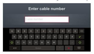
Entering the cable number as accurately as possible makes it easier to assign the cable later when reporting and archiving the measurement data record in the reporting software. If this kind of further processing is not planned, the cable number does not have to be entered. Regardless of whether or not a cable number has been entered, confirmation via vis required.
