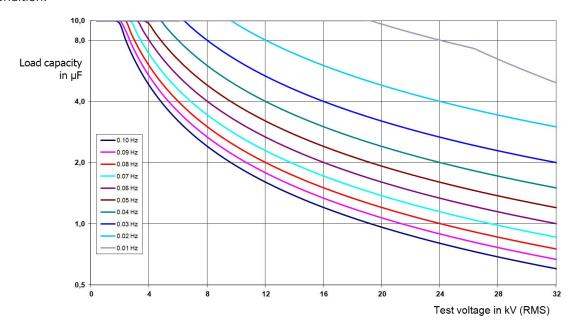
For **cosine rectangular voltage and damped AC voltage (DAC)** (boost module required), the following load diagram applies as and where appropriate <sup>1</sup>:
