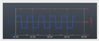
In DC mode, from a test time of approximately 90 seconds, a red arrow is also permanently displayed in the graph, showing the trend of the measured leakage currents (current measured value compared to the value measured after the charging process has been completed).
