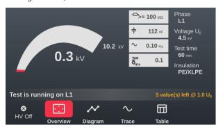
In addition to the current test voltage and the remaining test duration (or the remaining measured values in the step test), this also displays the following measured values:
