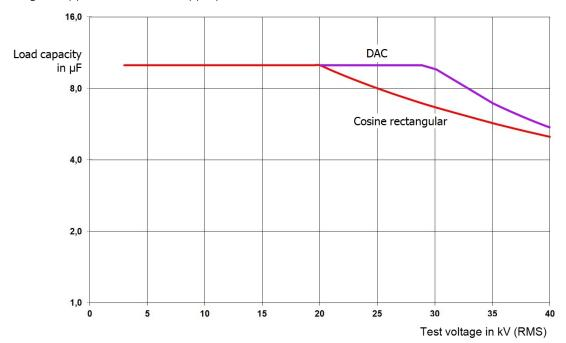
$<sup>^{1}</sup>$ Only valid between -25 and 45°C. In the temperature range from 45°C to 55°C, the power is reduced to 80% at 40 kV.
