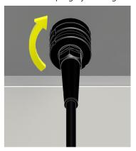
5. Secure the plug of the supplied HV connection cable to the HV output 17 of the boost module. Once again, you must ensure correct alignment when inserting the plug.
