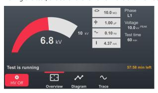
In addition to the current test voltage and the remaining test duration, this also displays the following measured values depending on the operating mode:
