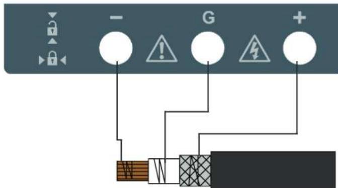
As illustrated in the diagram, the guard terminal is at the same potential as the negative terminal. Since the leakage resistance is effectively in parallel with the resistance to be measured, the use of the guard causes the current flowing through surface leakage to be diverted from the measuring circuit. The instrument therefore reads the leakage of the insulator, ignoring leakage across its surface.
