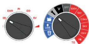
A timed test IR(t) will automatically terminate an insulation test after a preset time. Default timer is set to 1 minute and is adjustable within the settings function. This is a useful feature which saves the user watching the display for the full duration of the test and the possibility of missing the 1 minute reading.
