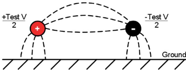
Conversely, if the positive terminal is grounded, then the negative terminal will be at a voltage equal to the test voltage relative to ground, which will result in an increase in leakage current, and worsening of measurement accuracy.
