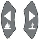
Left and right arrow buttons toggle between burn and breakdown mode when a voltage range is selected. Press and hold left arrow / burn to activate burn mode.
