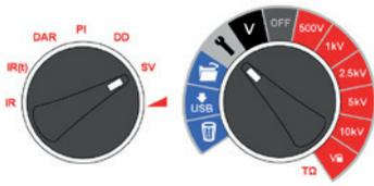
The SV test is a controlled overvoltage test that can be applied to stator and rotor windings on synchronous and asynchronous AC motors and the armature and field windings on DC motors. It is advisable to perform a PI test before an SV test to determine if the insulation is suitable for overvoltage testing. If a PI test was performed to verify the winding's suitability for over voltage testing, the winding must be completely discharged before the overvoltage test is performed.
