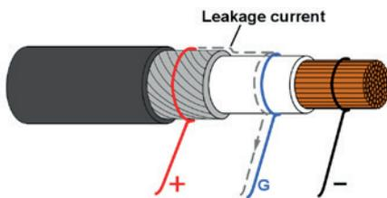
This diagram illustrates GUARD terminal used to prevent surface leakage on cable insulation from affecting a high resistance measurement.
