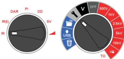
To set the clock and date, select the settings function on the central rotary switch and turn the mode rotary switch to IR. Navigate using the left / right arrows to where the time and date is displayed.
