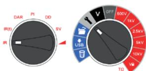
To set the user defined lock voltage  $V_{\text{L}}$ , turn the central rotary switch to settings and the mode switch to IR. The preset voltage 5000 V will flash and can be changed using the up / down buttons. When the required maximum voltage is displayed, press the OK button to save the setting. This setting will remain until it is reset.
