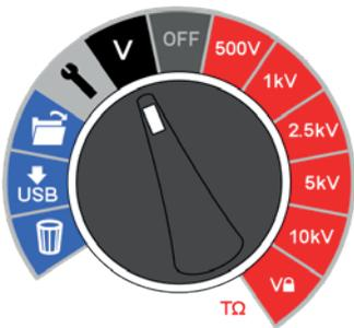
To assist user safety, the instrument will automatically switch to voltmeter mode if a voltage of 50 V or more is connected to the terminals. The measured voltage will be displayed accompanied by an intermittent beeper to warn the user that a dangerous voltage exists.
