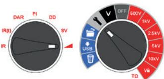
The ramp voltage test is an overvoltage test similar to the SV test but with improved control and warning of potential insulation failure. The slow continuous voltage ramp is less likely to result in unpredictable damage to the insulation than the rapid step increases employed in SV test.
