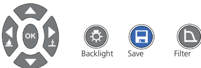
Four arrow buttons and OK facilitate adjustment and selection of settings, voltages and modes. Breakdown / burn modes are set using the left and right arrow buttons. Back-light and save functions are dedicated buttons. All models have backlight and the MIT525, MIT1025 and MIT1525 have the Save button.
