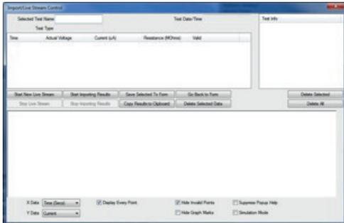
Import / Live Stream Control application enables capture of live streaming data directly by activating the Start New Live Streaming function. Results are recorded once a second for the duration of the test.
