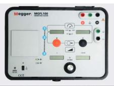
Connect the red terminal to the positive side of the battery string.
