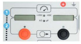
Once the transmitter had completed booting up the lower left voltage display will be flashing.
